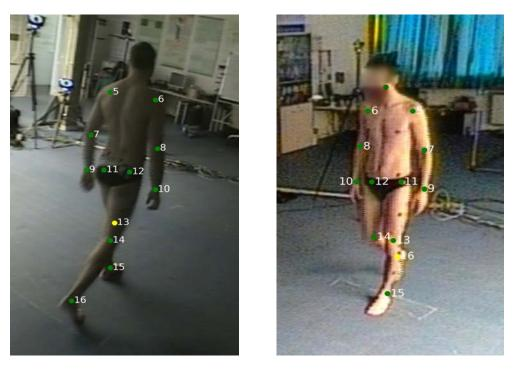
Figure 4.10: 2D pose estimates generated by HRNet from two views of walking subjects in an OW environment.
