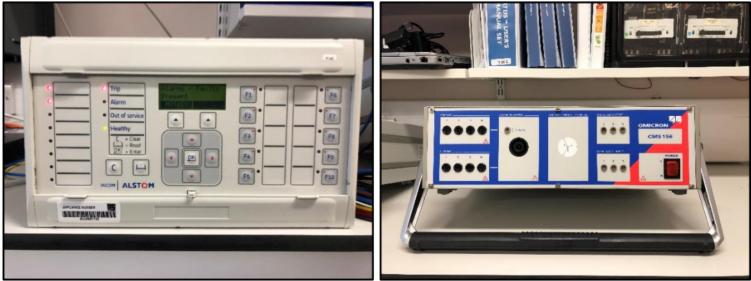
Fig. 13.2 Overcurrent relay and amplifier
