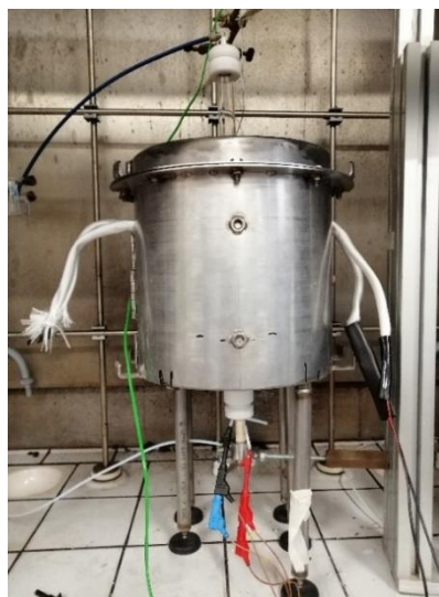
Figure 2.6. Electrical oven used to reach the operating temperature of 650^{\circ}\text{C} .
