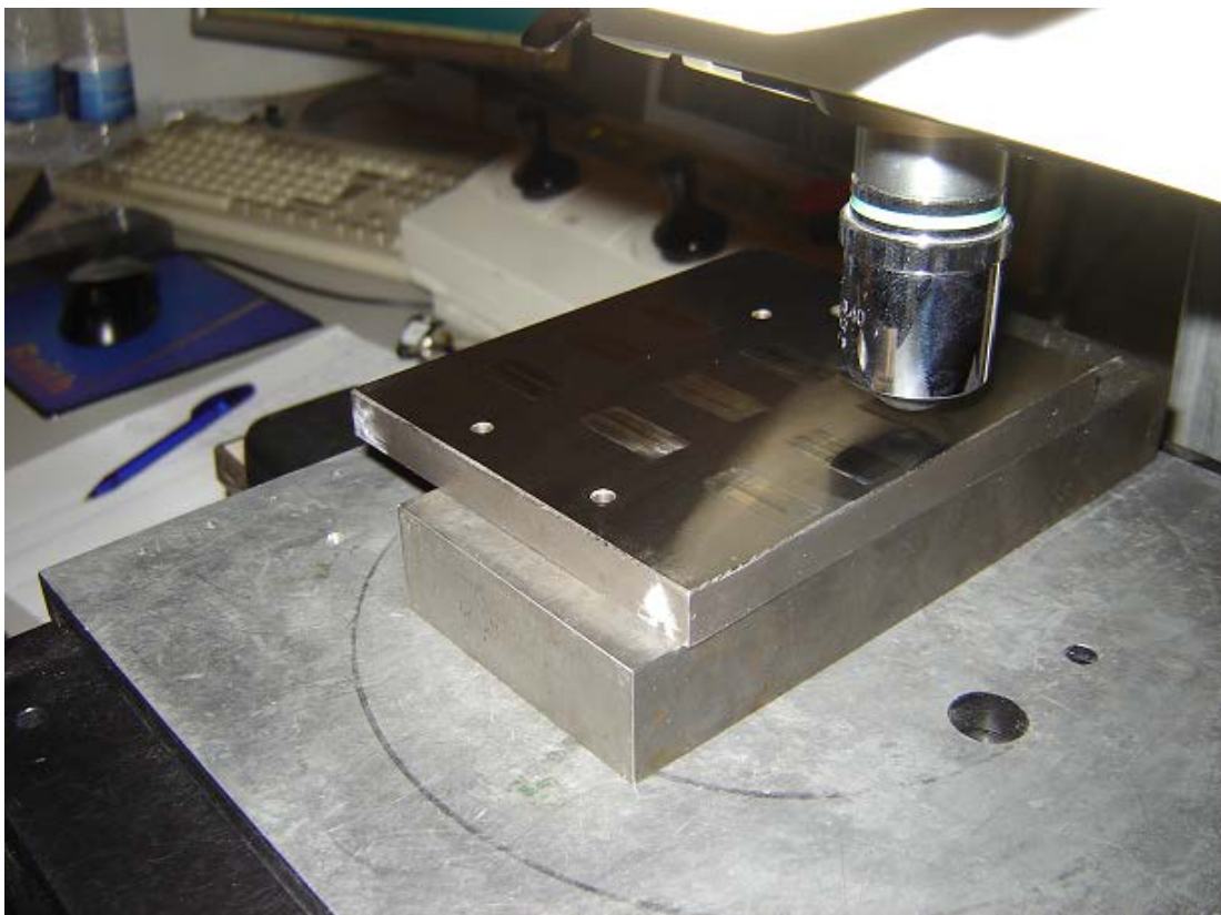
FIGURE 5.14 Measurements of polished surface with WLI
