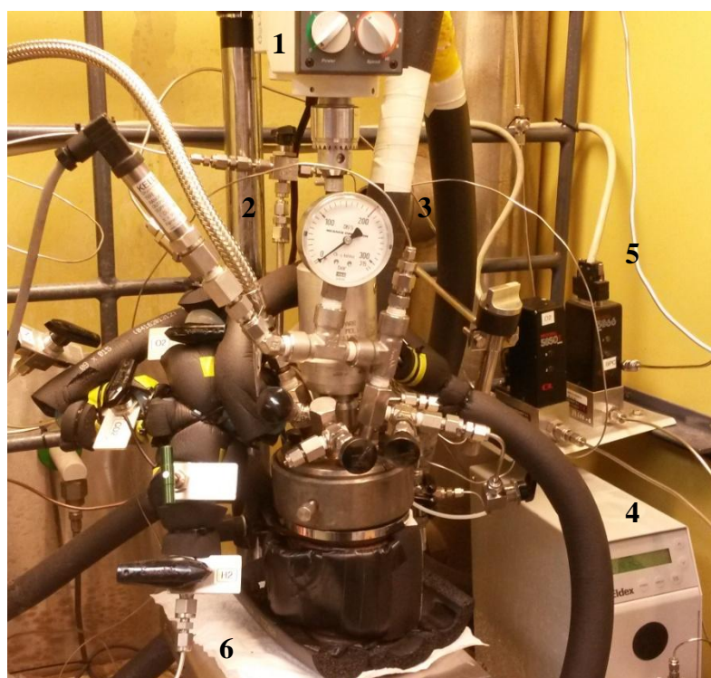
Figure 2.8. View of the semibatch apparatus. It is recognizable: 1- Agitator motor; 2 – Injection chamber; 3 – Condenser; 4 – High pressure pump; 5 – Flow mass controller; 6 – reactor and cooling jacket fitted in an isolating cover. On the left of the reactor, the on-off valves for the gases introduction appear. Between the pump and the reactor there is the 6-ways valve for the liquid sampling.
