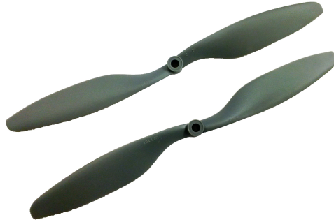
Figure 2.9 – Propellers of the quadcopter, puller on the top and pusher on the bottom.
