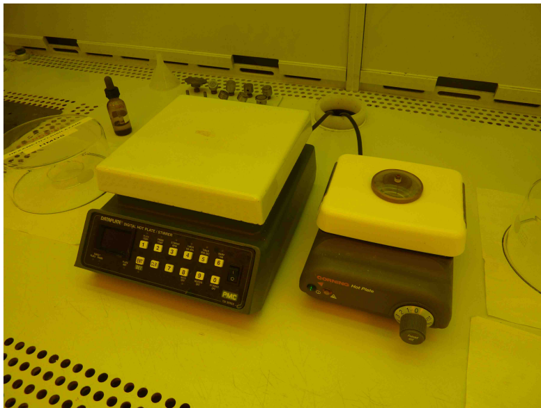
Figure 4.6: Hot plate for pre exposure softbake and post exposure bake.
