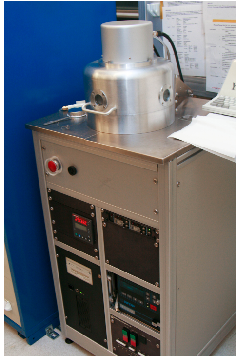
Figure 4.18: PECVD Plasma Therm 790 for Oxides and Nitrides deposition.
