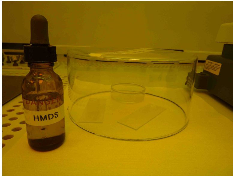
Figure 4.4: HMDS treatment used to improve the adhesion of photoresist.
