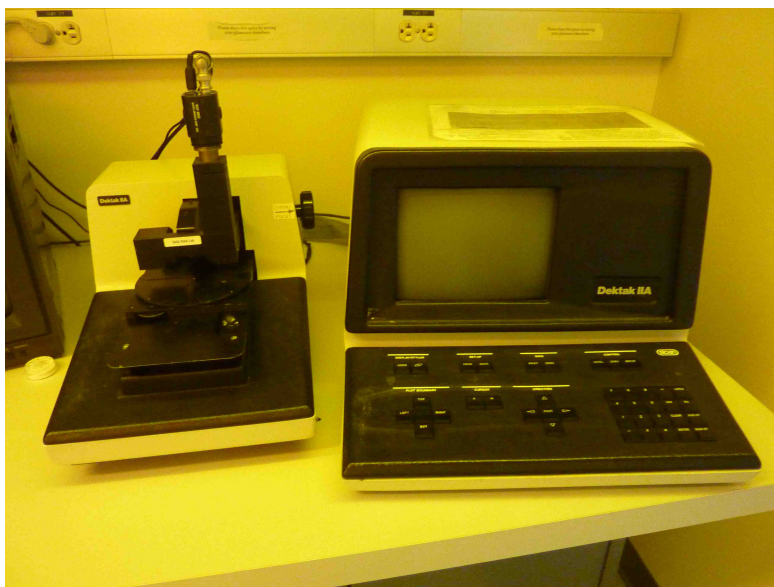
Figure 4.8: Dektak profilometer used in the test step.
