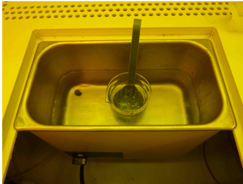
Figure 4.3: Ultrasonic cleaner used in the standard cleaning procedure.
