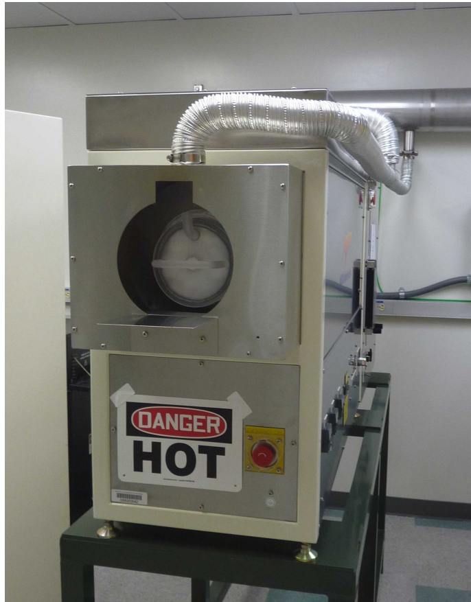
Figure 4.15: Furnace used to grow thermal oxide on a silicon wafer.
