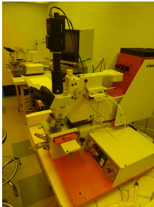
Figure 4.7: Karl Suss MJB3 mask alignment used in the lithography process.
