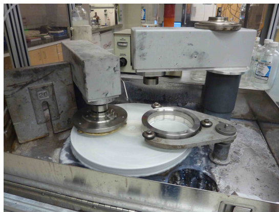
Figure 4.20: Lapping machine used during CMP procedure.
