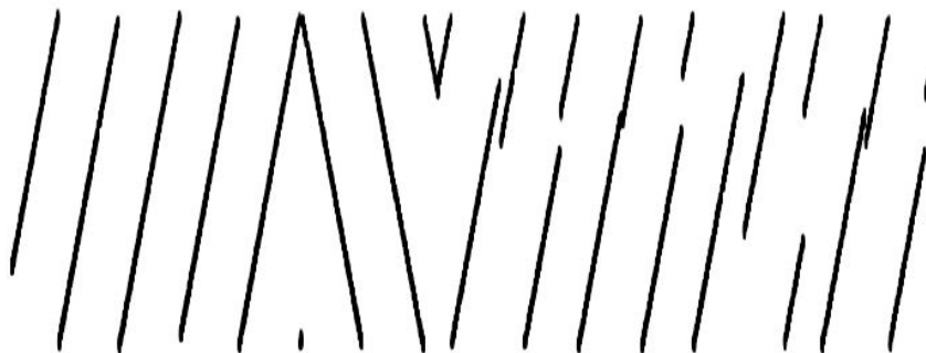
Figure 3.1: Spectrogram of a LoRa packet [6].
