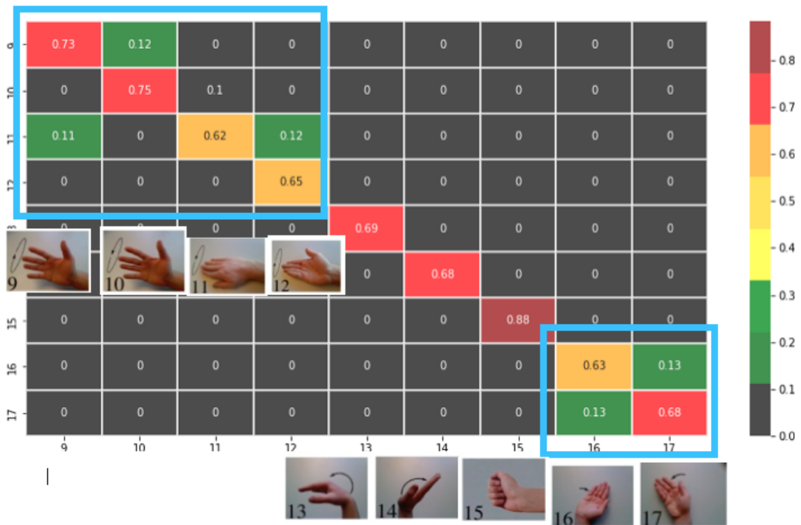
Figure 4.4: Confusion matrix for the RF working with the second subset of gestures.
