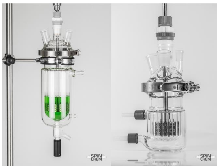
Figure 2.1. A SpinChem® RBR S311 placed in a 1200 mL vessel (on the left) and a SpinChem® RBR S221 in a 210 mL vessel (on the right).
