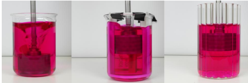
Figure 4.16. Influence of the baffles on the dimension of the vortex which is formed when the RB is rotating.
