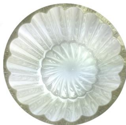
Figure 2.2. The interior of a flower-baffled vessel with eighteen baffles from the top.
