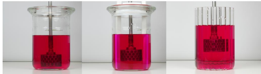
Figure 4.15. Set-up of the various experiments made with vessels of different diameter and different types of baffles.
