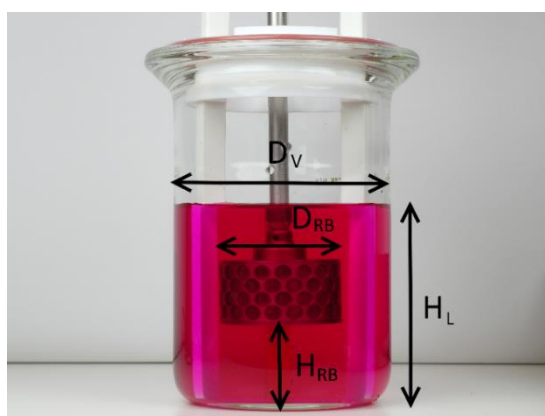
Figure 4.6. Main geometrical parameters of the reactors used.
