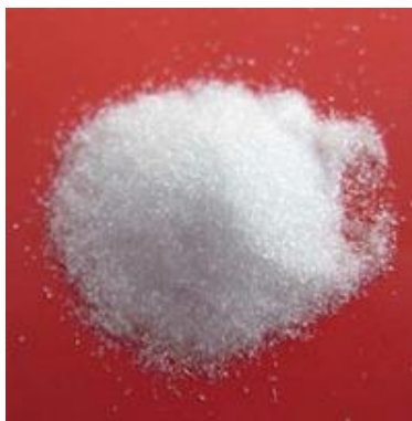
Figure 3.10. A picture of the thiol scavenger SiliaMetS® Thiol from SiliCycle used (particle size = 200-500 \mu\text{m} ).
