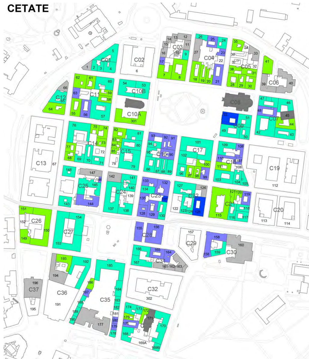
Fig. 6.6.2: Vulnerability assessment of PL2 - simple overturning mechanism
