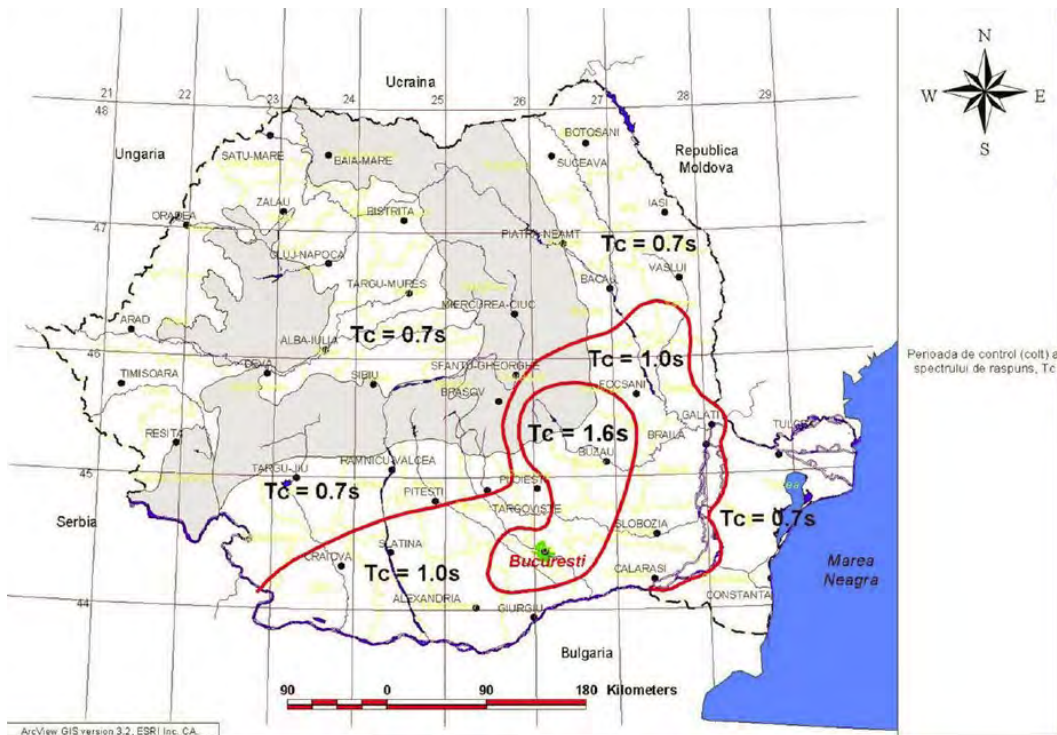
Fig.3.1.7: Romania in terms of zoning control period (corner), T_c response spectrum. Code design P100-1 / 2006
