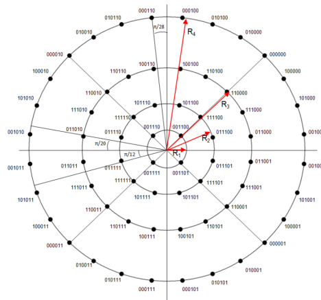
Figure 2.12: Example of 4+12+20+28APSK constellation
