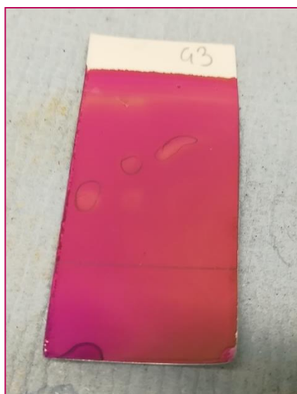
Figure 6.27. TLC paper in benzene:methanol (95:5) eluent. The three separated references for guaiacol, creosol and 4-ethylguaiacol are circled with a pencil.
