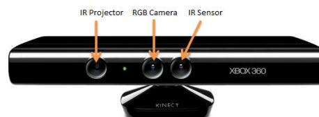
Figure 3.1: Components of the Kinect sensor: ir projector-sensor and RGB camera.
