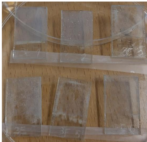
Figure 44 - Picture of the samples in batch 3. Except for the first and the second, they show irregular surfaces, where many spots look more transparent because the growth of NWs was occasionally unsuccessful.
