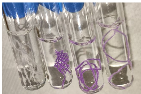
Fig. 32: Schiff test with the fresh Schiff reagent on A-cotton. From the left: A-cotton, 1 st oxidation of A, 2 nd oxidation of A, 3 rd oxidation of A.
