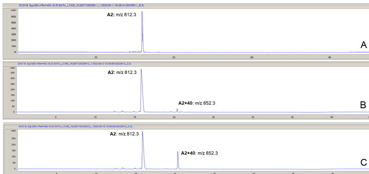
Fig. 38: LC-MS monitored at 280 nm of the A2 fraction after the purification, (A) Immediately after the purification; (B) The day after the purification. Solution stored in the fridge; (C) The day after the purification. Solution used for measure A, kept out of the fridge for the night.
