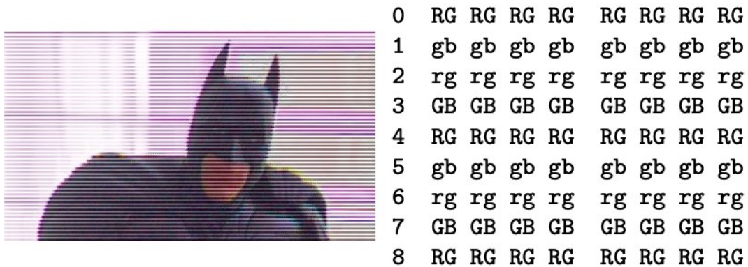
Figure 8.3 – Resulting interlaced image (left) and the alternated Bayer pattern (right) [38]
