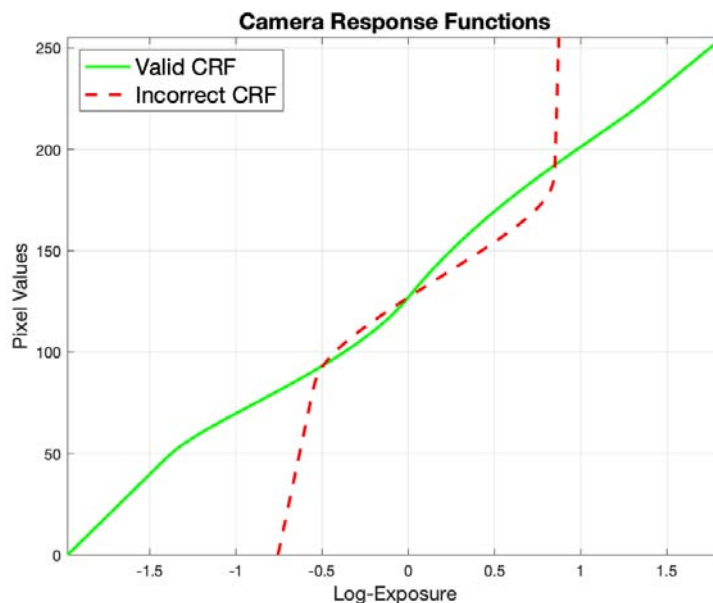
Figure 8.1 – CRF computed from still pictures compared with a visibly wrong CRF obtained with a dynamic subject
