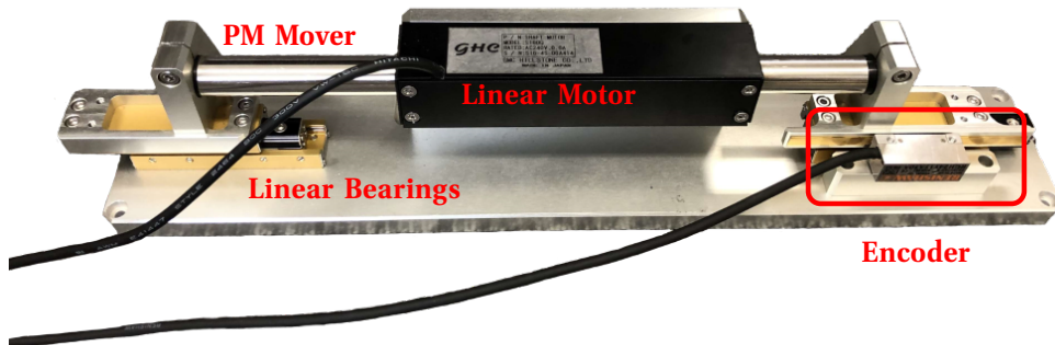
Figure 8: Experimental setup: linear motor and position encoder.
