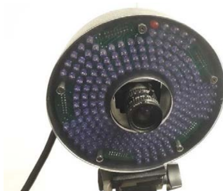
Figure 2.4: One of the infrared cameras of the Motion Capture system.
