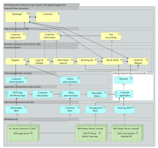
Figure 5. Target architecture for the integration of the sales area/fare management of the BerlKönig service
