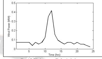
Figure 3. Wind power profile for single day
