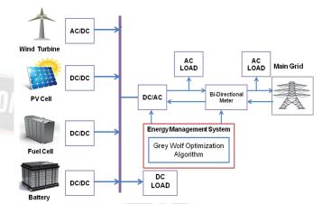
Figure 1.Structure of proposed microgrid system
