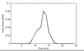
Figure 2. Solar power profile for single day
