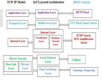
Figure 3. The Layered Architecture of IoT.
