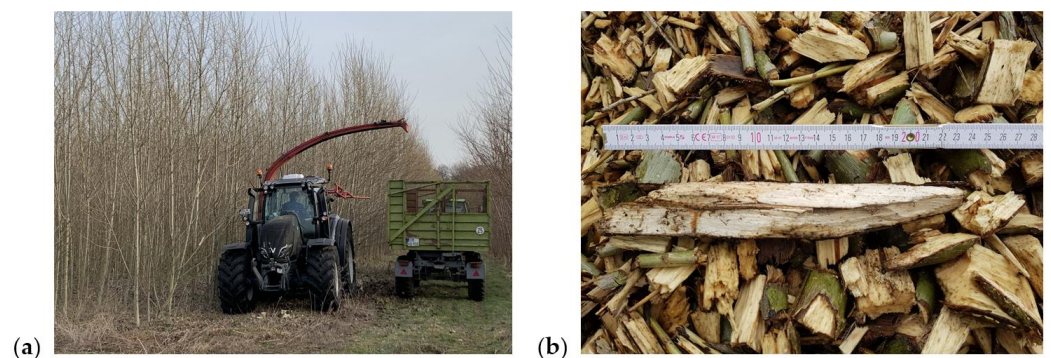
Figure 1. (a) Harvest of poplar with a mower-chipper. (b) Wood chips produced at harvest.
