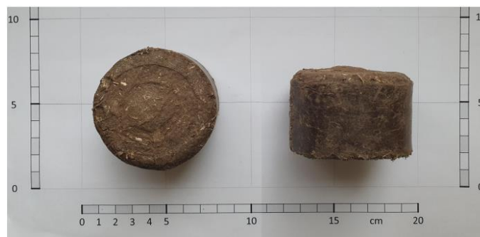
Figure 3. Dimensions of the briquettes produced from poplar fibre.
