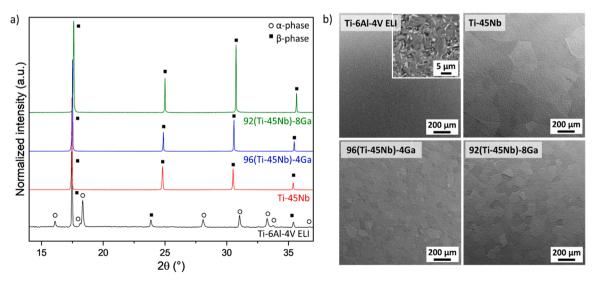
Fig. 2. (a) XRD diffraction patterns and (b) SEM micrographs of investigated alloys.
