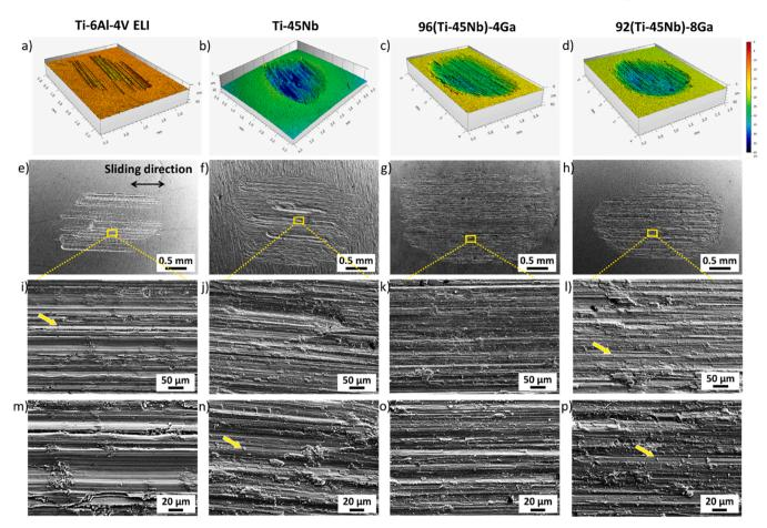
Fig. 6. Morphological features of the wear tracks under OCP conditions of the four tested alloys characterized by (a-d) 3D optical profilometry and (e-p) SEM. Squares in e-h represent areas of interest shown in i-p (sliding direction, valid for images e-p, is indicated by double arrow in image e). (For interpretation of the references to color in this figure legend, the reader is referred to the web version of this article.).
