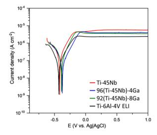
**Fig. 3.** Potentiodynamic curves recorded at a scan rate of 0.5 mV/s of the four alloys in PBS solution after OCP adjustment of 3600 s (For interpretation of the references to color in this figure legend, the reader is referred to the web version of this article.).
