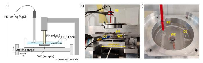
Fig. 1. (a) Scheme of the tribo-electrochemical setup, (b) side view and (c) top view (without pin holder).
