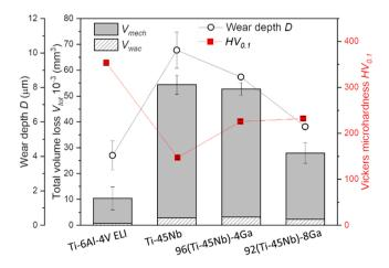
**Fig. 7.** Variation per alloy of total volume loss ( $V_{tot}$ ) with the contributions of mechanical wear ( $V_{mech}$ ), wear-accelerated corrosion ( $V_{wac}$ ) and wear depth (*D*) measured by 3D optical profilometry, plotted with Vickers microhardness ( $HV_{0,1}$ ).
