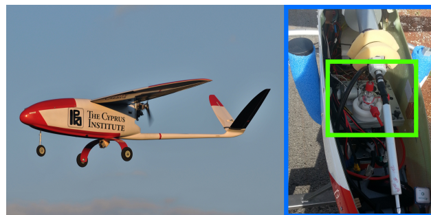
Figure 6. The Cruiser UAS with the multi-sample aerosol collector (green rectangle; photograph by Kjell-Sture Johansen).
