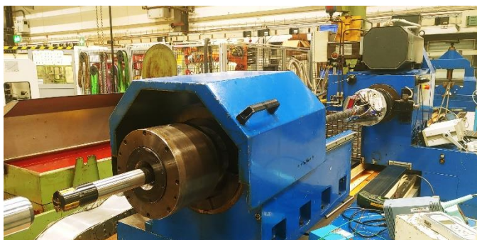
Fig. 2. Giana GGB560 BTA deep hole drilling machine (blue) with mounted CFRP drill tube, drill head (left) and the sensor platform
