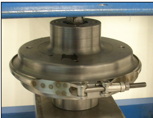
Figure 1: V-section band clamp assembled to a pair of circular flanges for initial experimental testing
