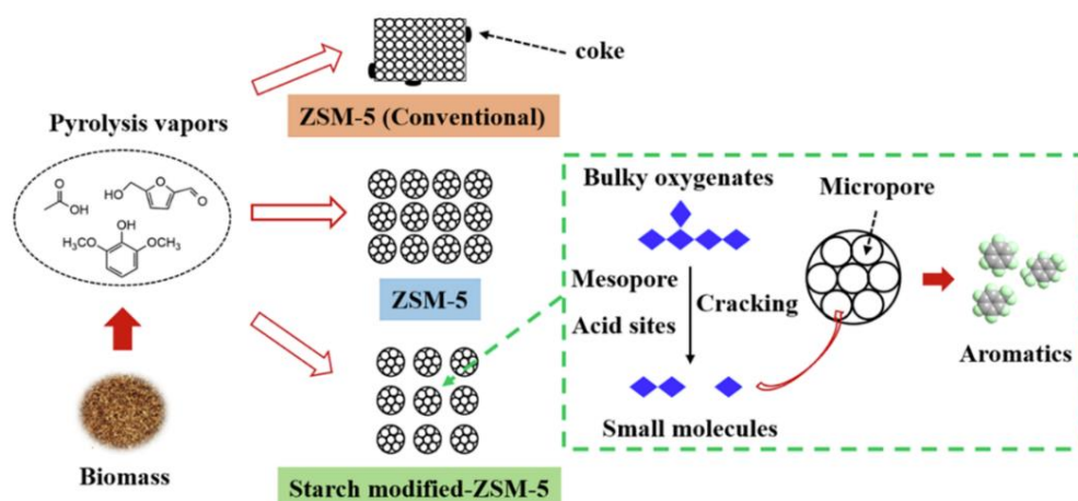
Figure 2 Illustration of the catalytic fast pyrolysis (CFP) of biomass over conventional zeolite vs. hierarchical zeolites. Reproduced with permission from Ref. [43]. © 2019 Elsevier.
