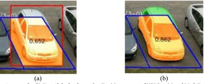
Figure 13. An example of IoR result by implementing Eq. (5) on output of YOLOv4 (a) and Mask R-CNN (b)
