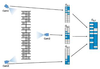
Figure 5. Information fusion example: parking and monitoring cameras (left), single-camera extracted occupation information (center) and result of the information combination (right). Courtesy of Nieto et. al. [18]
