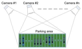
Figure 6. Arrangement of surveillance cameras in our scenario
