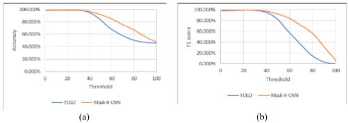
Figure 12. Performance analysis of YOLOv4 and Mask R-CNN on CNRPark-EXT dataset (a) accuracy and (b) F1 score
