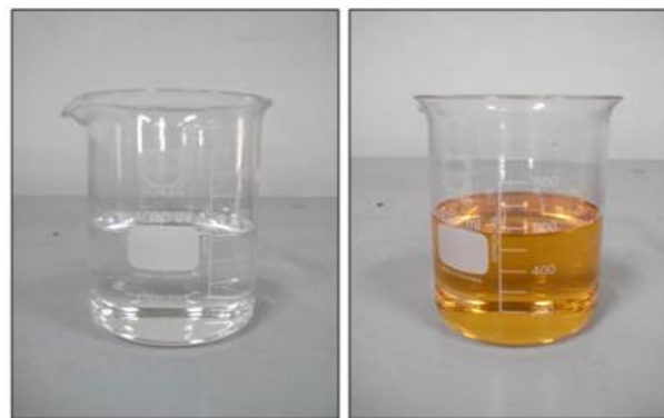
(a) Mineral oil (b) olein-sawn oil Figure 4. Oil samples for electrical insulation
