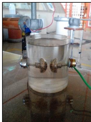
(a) High voltage test circuit (b) The test cell contains the oil to be tested Figure 6. Circuit for testing the breakdown voltage of the palm oil-ester sample
