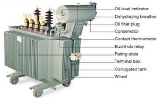
Figure 2. Electric power transformer and its parts
