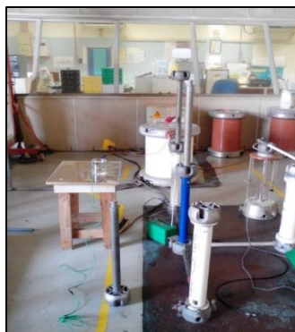
(a) High voltage test circuit (b) The test cell contains the oil to be tested Figure 6. Circuit for testing the breakdown voltage of the palm oil-ester sample
