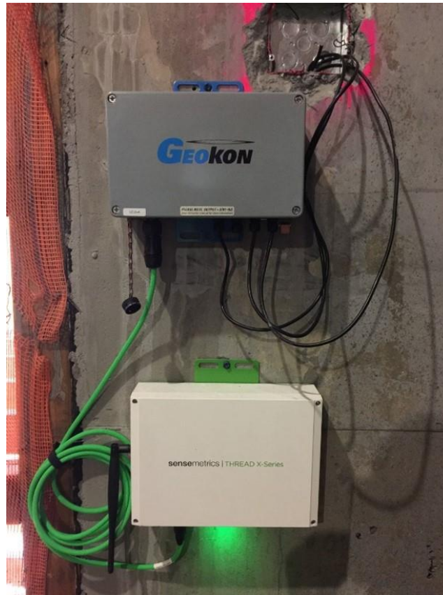
Figure 5.3 Geokon Datalogger and Sensemetrics Thread.
