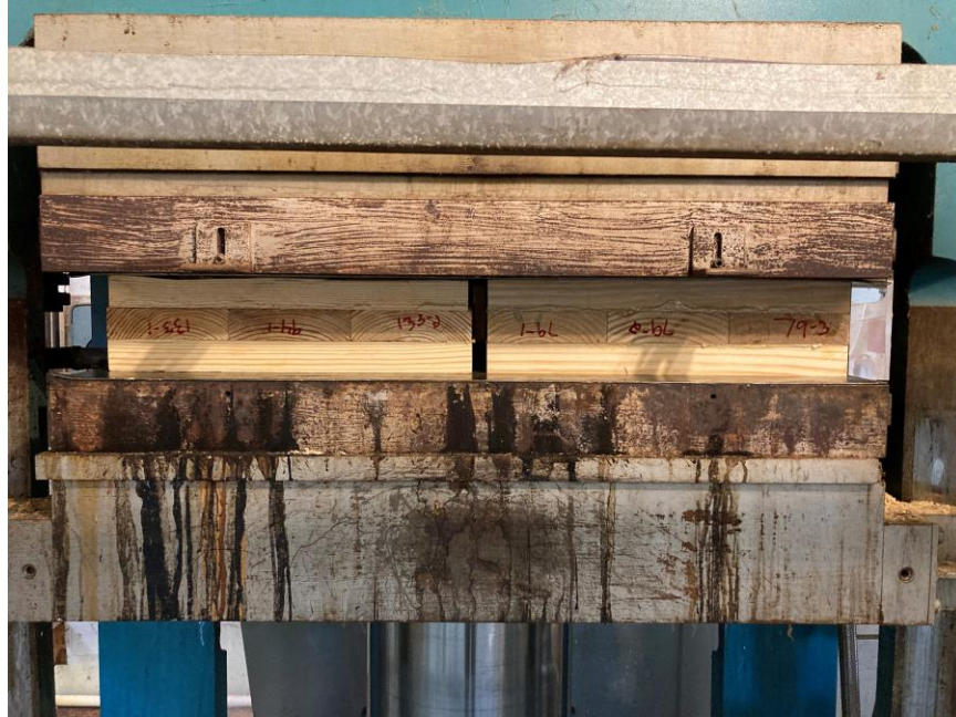
Figure 3.2 3-ply CLT panels in Dieffenbacher laboratory hydraulic press
