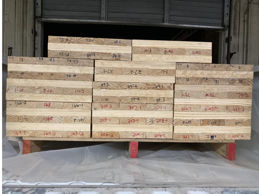
Figure 3.3 Eleven CLT panels ready for transportation to Deforest Wood Preserving in Bolton, MS for CA-C treatment
