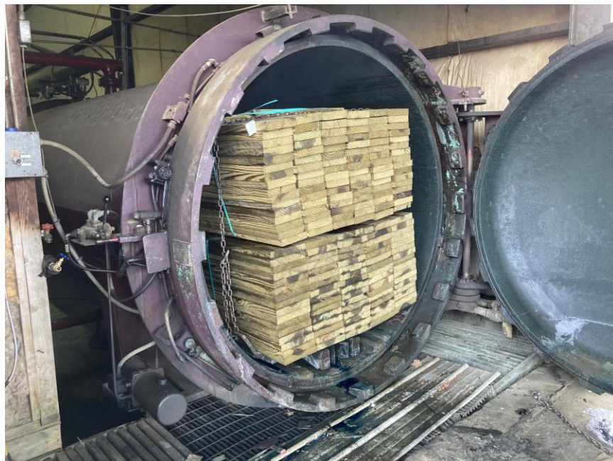
Figure 3.4 Charge of lumber coming out of treatment cylinder at Deforest Wood Preserving. CLT samples at the other end of treatment cylinder
