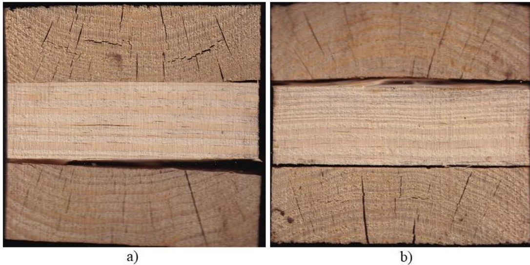
Figure 3.31 Wood laminates after accelerated weather cycles: a) dimensional changes out of plane and b) dimensional changes in-plane
