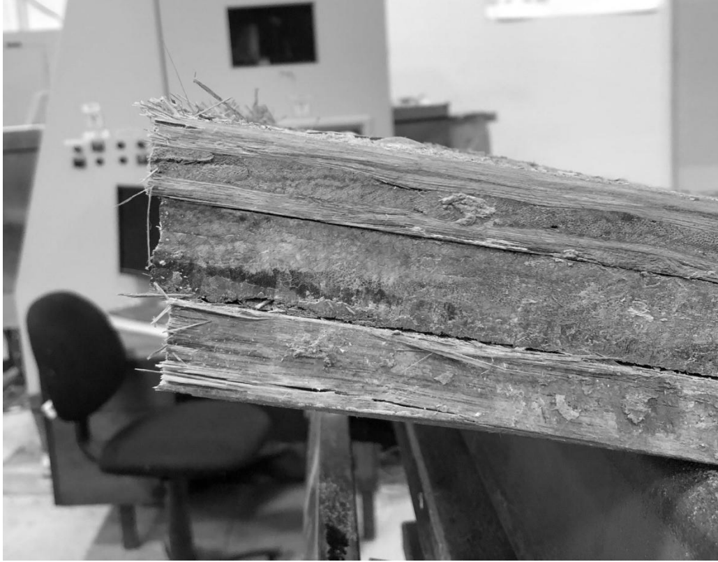
Figure 4.7 The end of an exemplar billet during mechanical testing; the sliding action of the three individual plies under flexural strain is visible
