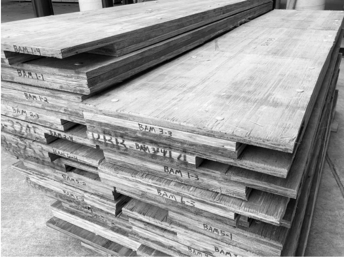
Figure 4.4 Stack of machined 3-ply bamboo billets staged for mechanical testing
