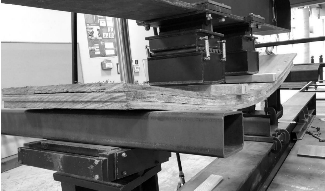
Figure 4.5 Exemplar picture of one billet during destructive flexural testing
