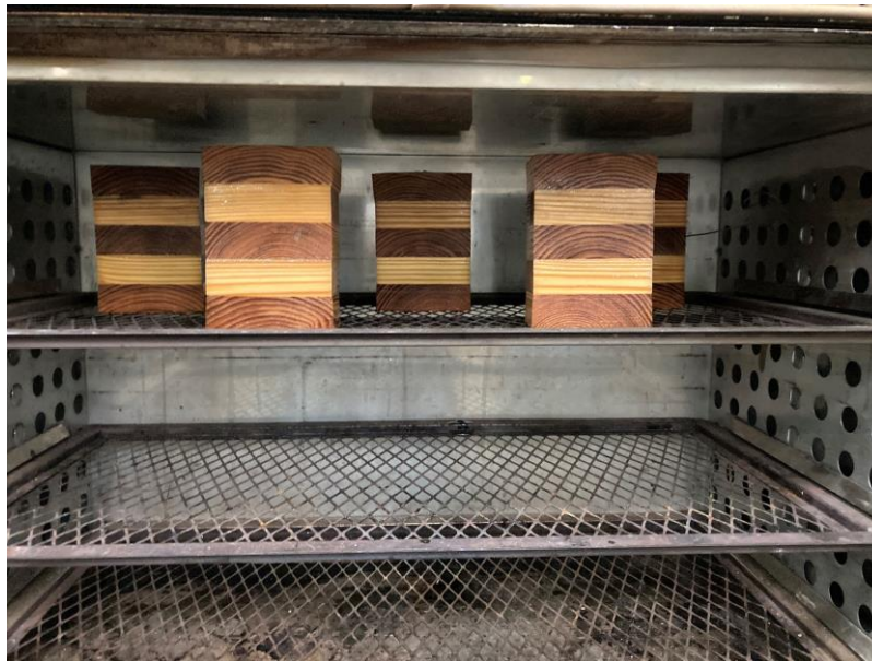
Figure 3.16 Oven-dry process for delamination test
