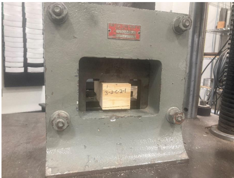
Figure 3.13 Block shear specimen in block shear set-up in Tinius Olsen Machine
