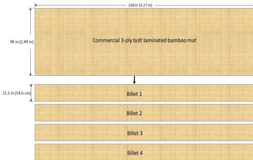
Figure 4.1 Four testing billets were cut from each 3-ply bolt laminated bamboo mat
