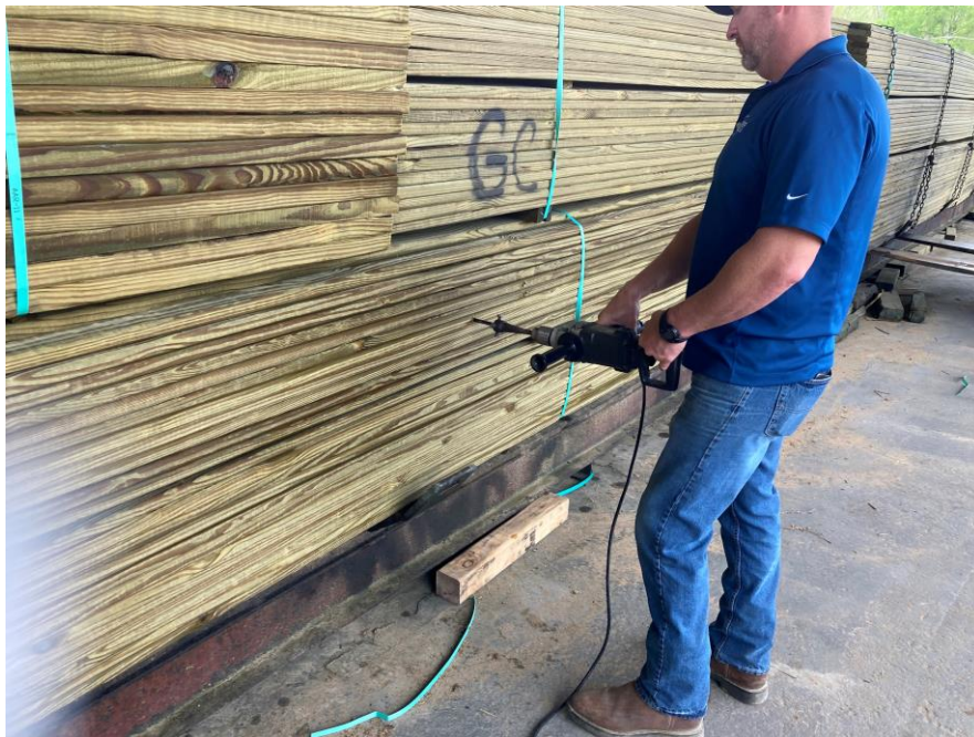
Figure 3.8 Mr. Jeremiah of Deforest Wood Preserving boring cores from lumber in charge to test for preservative retention
