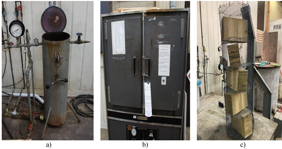
Figure 3.14 Delamination test equipment: a) pressure vessel; b) blue m oven; c) samples in wire mesh basket
