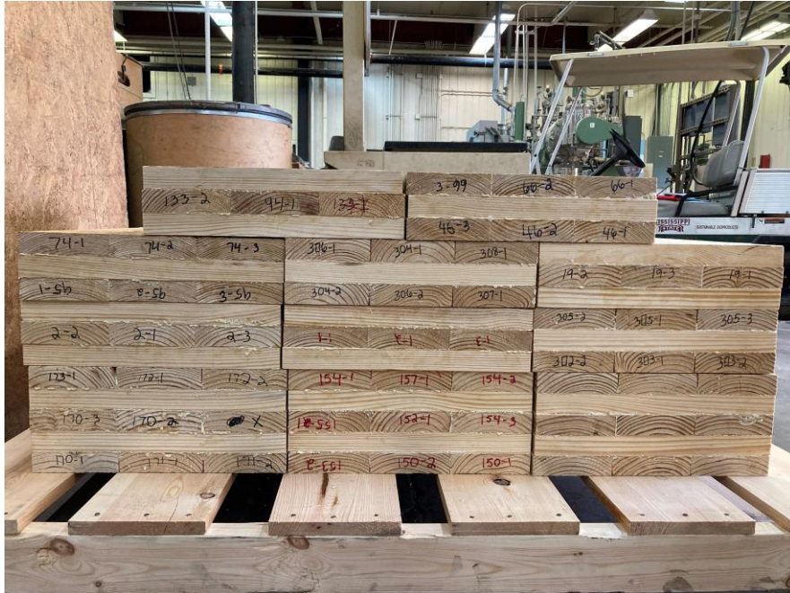
Figure 3.6 CLT panels prepared for shipment to Koppers Performance Chemicals in Griffin, GA for MCA treatment
