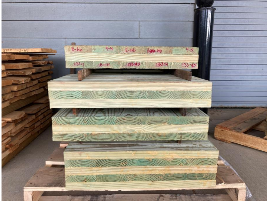
Figure 3.7 CLT panels after MCA treating at Koppers Performance Chemicals
