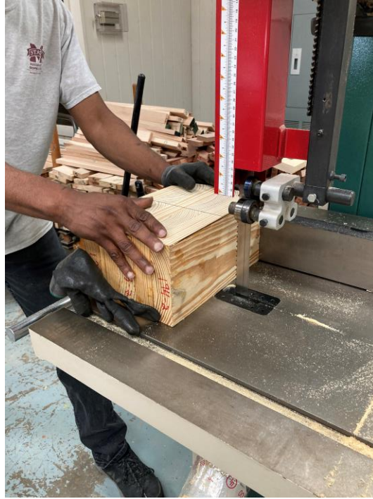
Figure 3.10 Cutting CLT panels into square blocks
