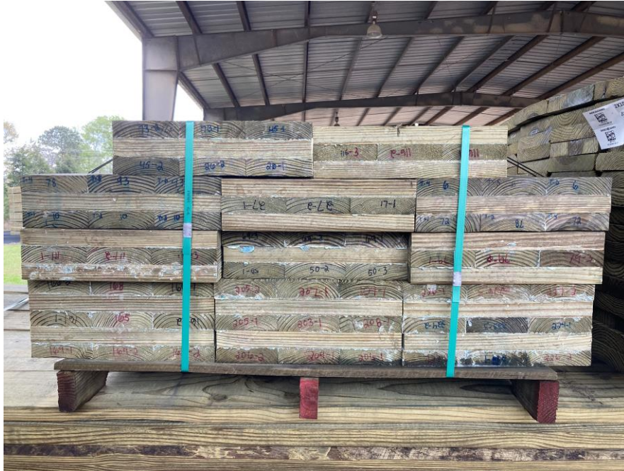
Figure 3.5 CLT panels after CA-C treating at Deforest Wood Preserving
