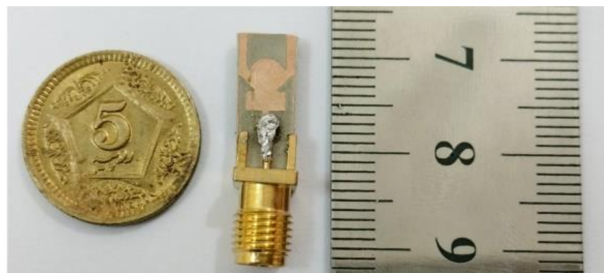
Figure 4. Fabricated prototype of wideband antenna.
