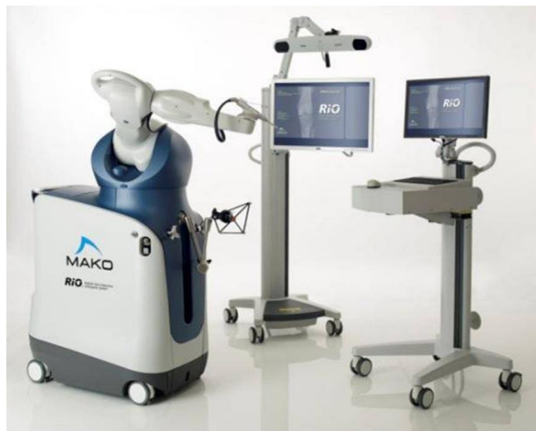
Figure 10. Photograph of the MAKO RiO System: haptic arm (left), the infra-red navigation camera (center), and the guidance module (right) (Stryker, 2017).
