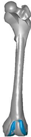
Figure 30. Femur model comparison showing GEBOD-scaled model (grey) overlaid on CT-derived model (blue) from SimTK dataset. GEBOD-scaled model is undersized by 35 mm.
