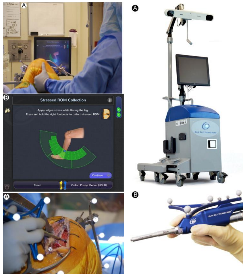
Figure 11. Navio Surgical System: the operative workflow (left), the cart and the navigation camera (right, top), and the robot-controlled burr (right, bottom) (Lonner and Kerr, 2012).
