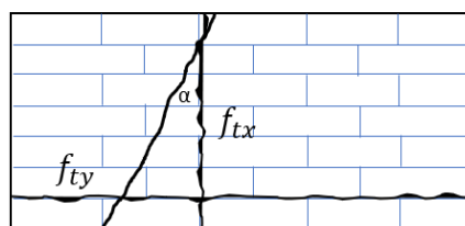
Figure 1. General characteristic of the Engineering Masonry model
