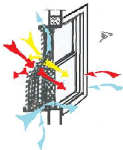
Figure 18. Schematic representation of established airflow between two wooden membranes of mušebak [47]
