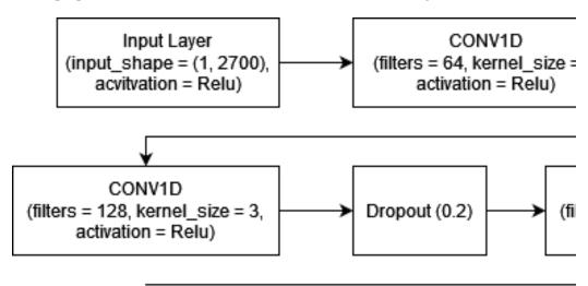
Fig. 3. Proposed 1 Dimensional CNN Architecture
