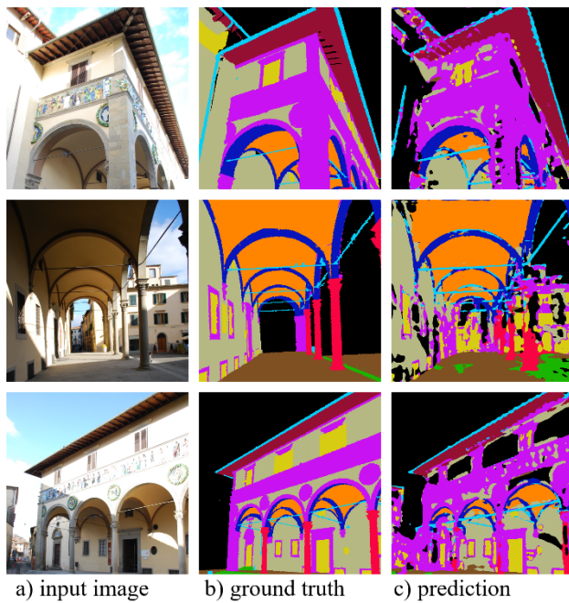
Figure 13. Test 2 – Prediction maps comparison with Deeplabv3+: a) input image, b) ground truth, and c) prediction.
