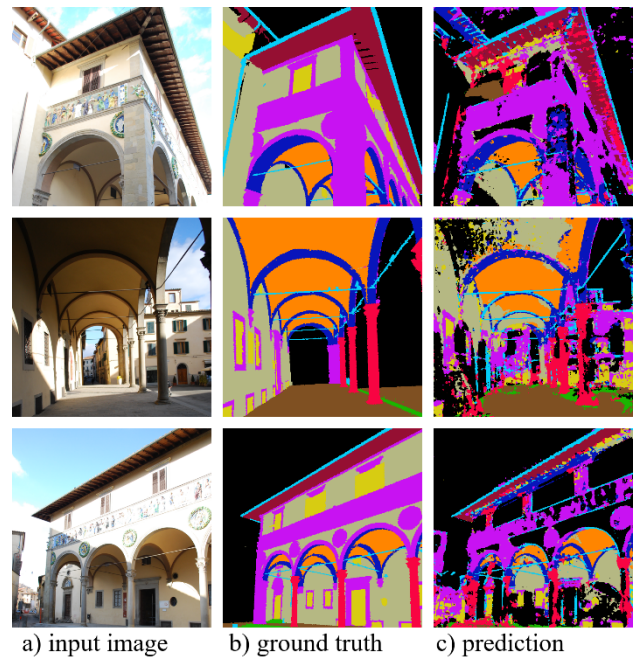
Figure 11. Test 2 – Prediction maps comparison with SegNet: a) input image, b) ground truth, and c) prediction.
