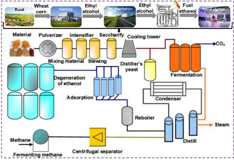
Fig. 13. Process of ethanol production from biomass fuel in Henan Tianguan Company
