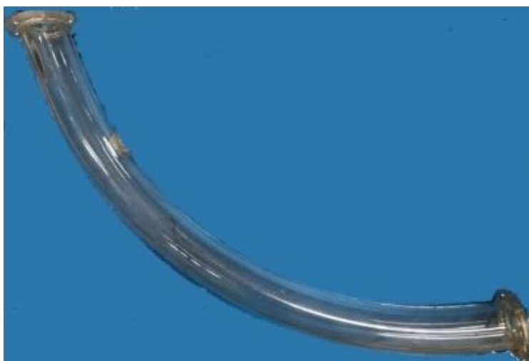
Figure-10: The pipe is made of transparent acrylic resin.
