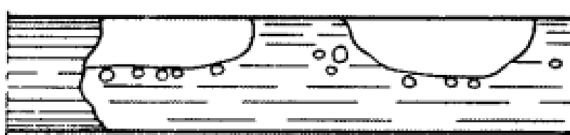
Figure-2: Plug flow structure [1]
