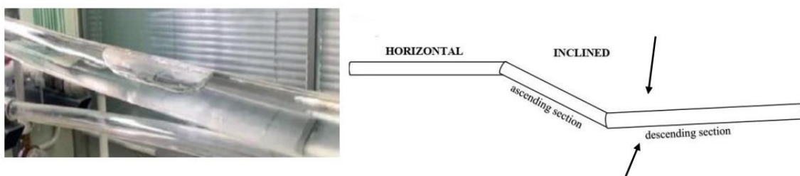
Figure-12: Structural flow of gas-liquid flow in the descending section of the pipe.
