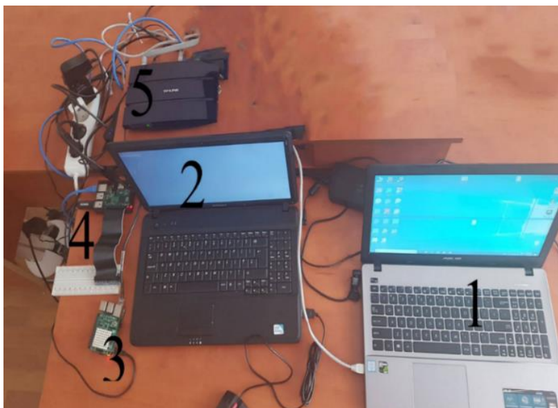
Fig. 4. Experimental scheme of the monitoring application: 1-Laptop; 2-Server equipped with Linux operating system; 3-RaspberryPi 3 sensors; 4-RaspberryPi 2 data bus; 5-Router.
