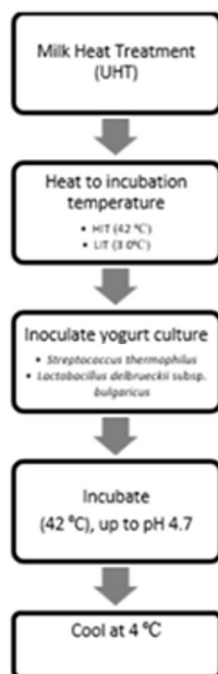
Figure 1. Scheme illustrating a method for yogurt production.
