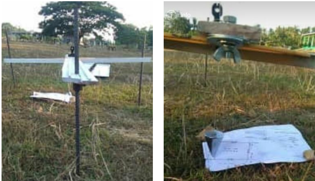
Figure 5. Locate the Point of Survey using Lot Sketch Plan and the Plumb bob
