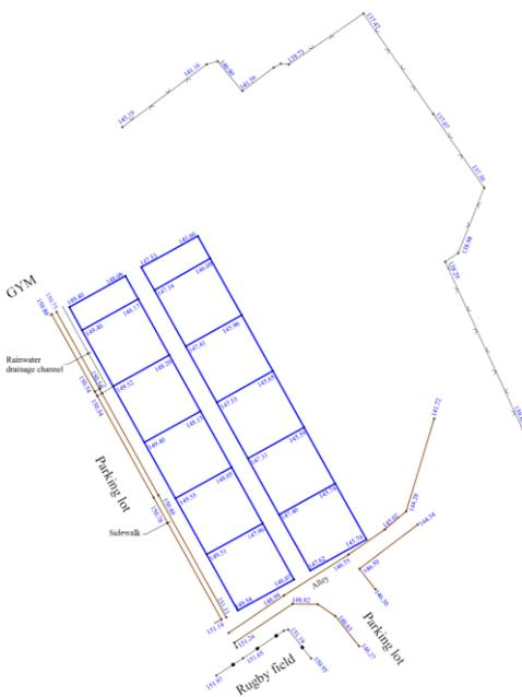
Figure 4 Application of geometric leveling with small squares
