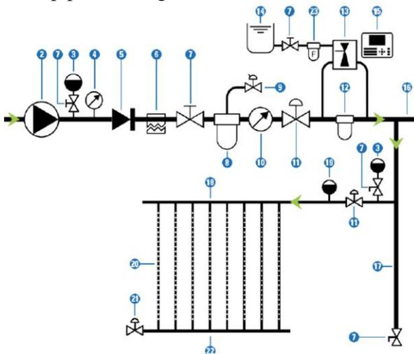
Figure 2 The structure of the drip irrigation system
