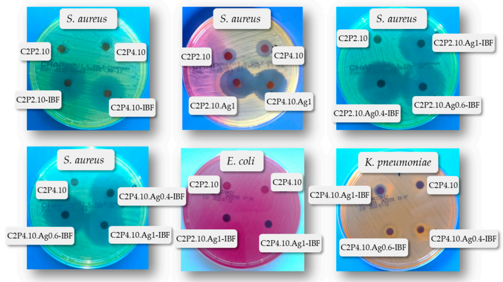
Figure 11. Antibacterial activity against S. aureus , E. coli and K. pneumoniae of film samples with and without the drug and with different percentages of AgNPs in the composition.
