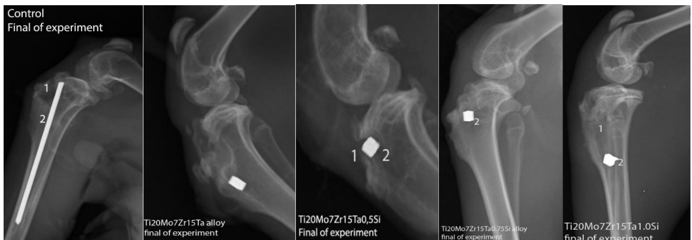
Figure 9. X-rays of control and experimental rabbits after 60 days of experiment, 1-alloy, 2-implantary breach.
