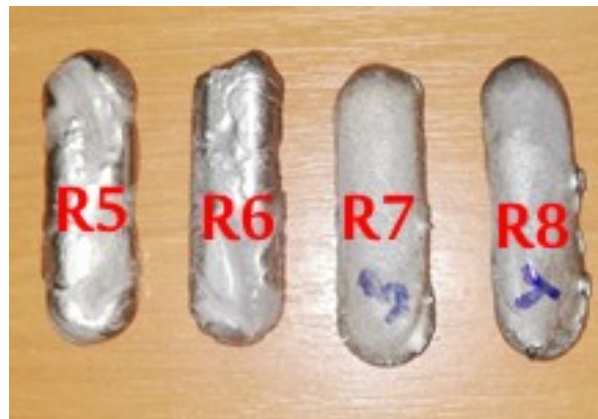
Figure 2. Mini-ingots of the alloys from TiMoZrTaSi system.
