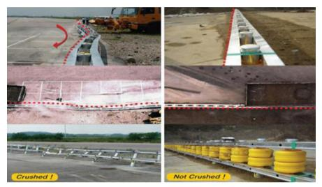
Fig. 9 - Crash test 1: comparison of traditional barriers and rolling barriers [20]
