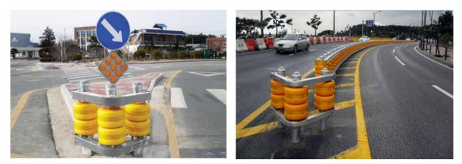
Fig. 5 - Median rolling barrier [11]
