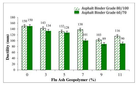
Fig. 4 - Relationship between fly ash geopolymer content and ductility for asphalt binder grade 80/100 and 60/70
