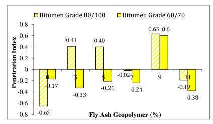
Fig. 3 - Effect of fly ash geopolymer on penetration index
