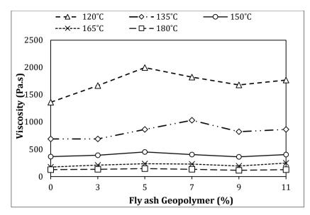
Fig. 7 - Relationship between viscosity and fly ash geopolymer content for asphalt binder grade 60/70
