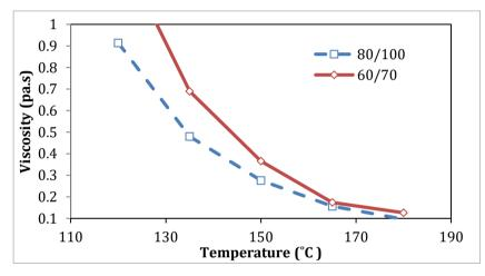
Fig. 5 - Viscosity versus temperature in asphalt binder grade 80/100 and 60/70
