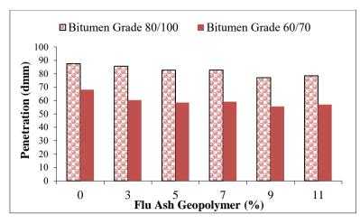
Fig. 1 - Relationship between fly Ash geopolymer content and penetration for asphalt binder grade 80/100 and 60/70
