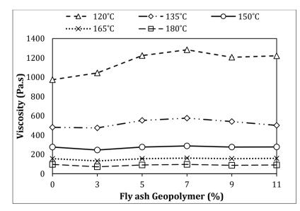
Fig. 6 - Relationship between viscosity and fly ash geopolymer content for asphalt binder grade 80/100
