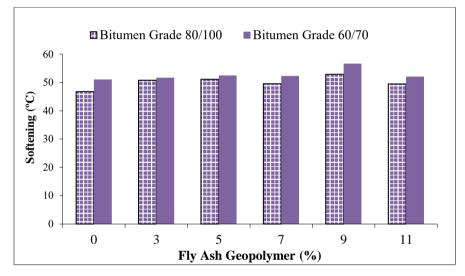
Fig. 2 - Relationship between fly ash geopolymer content and softening point for asphalt binder grade 80/100 and 60/70
