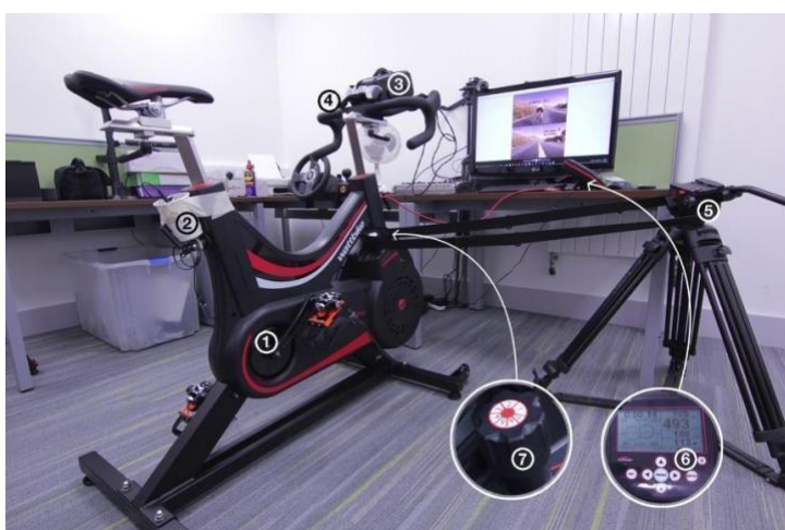
Figure 5.3: (1) Wattbike, (2) Arduino Wireless Heart Rate Receiver, (3) Oculus Rift, (4) Gamepad, (5) Resistance Pulley, (6) Wattbike Display Unit, (7) Resistance Dial.
